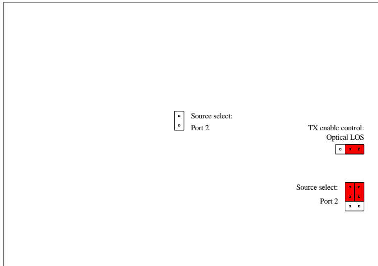
Figure 3: Jumper configuration for port 2 RX (default)
